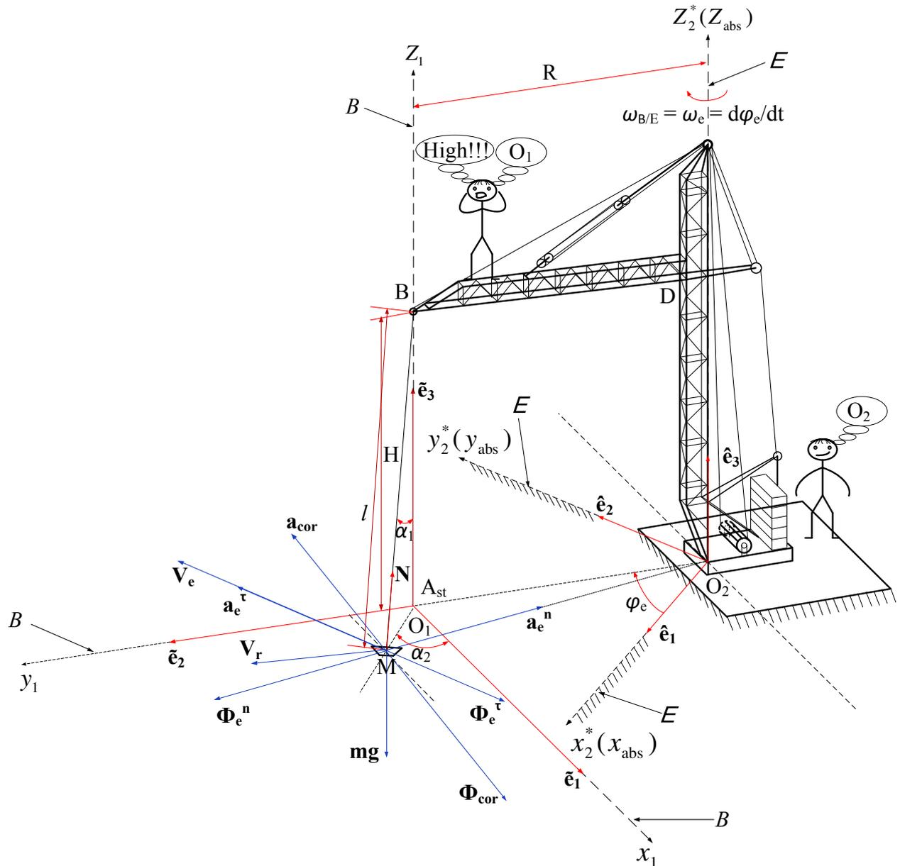
Figure 3. Computational scheme, illustrating concepts of Foucault pendulum-like systems in mechanical engineering problems of boom crane dynamics and control
